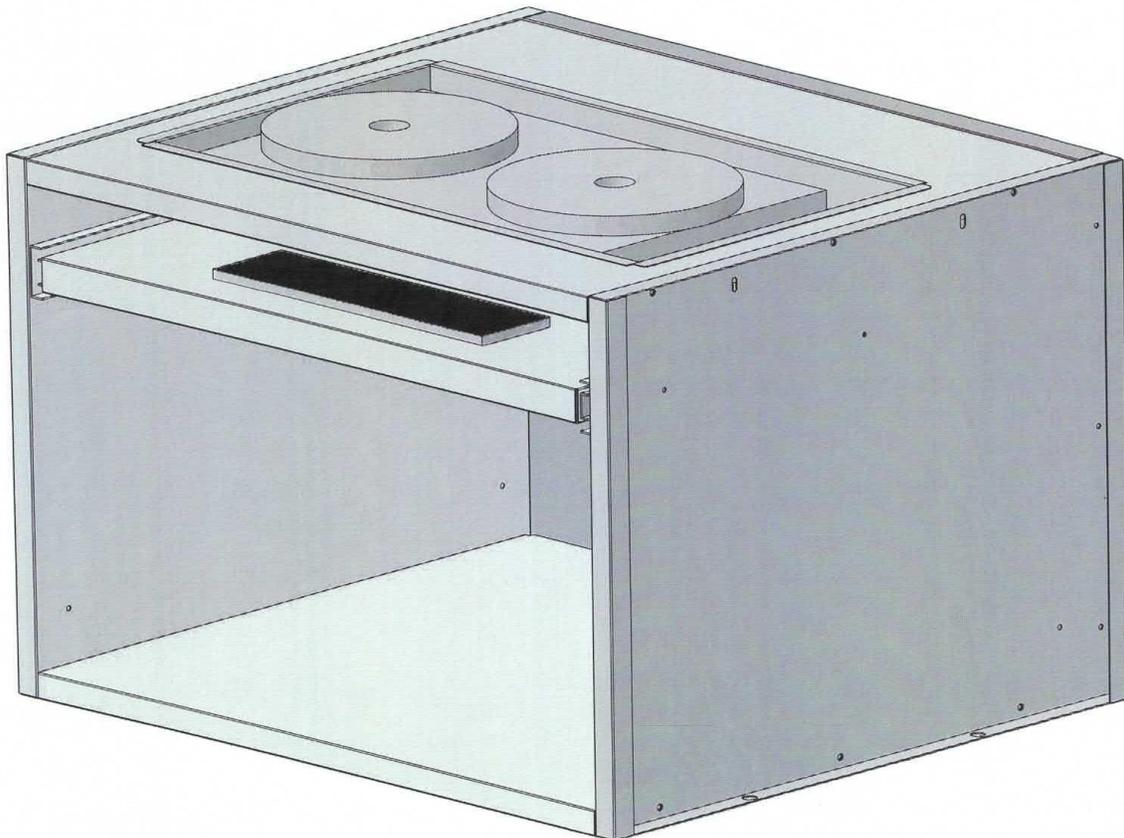
Drawer Size option depending on Cabinet width, with hole cutout size to drop in Controller in 15cm drawer or bottom of existing drawer
